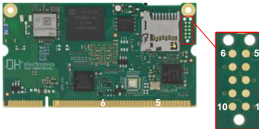
Figure 4: TAG Connect pin assignment on the topside of the DHC0M i.MX8M Plus to use with a TC2050-IDC-NL cable
